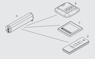
The 5100TC is supplied with a remote control and a timer unit to give total control.
