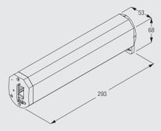
The motor 5190 is supplied with a 5m power cable with a 3 pin plug.
